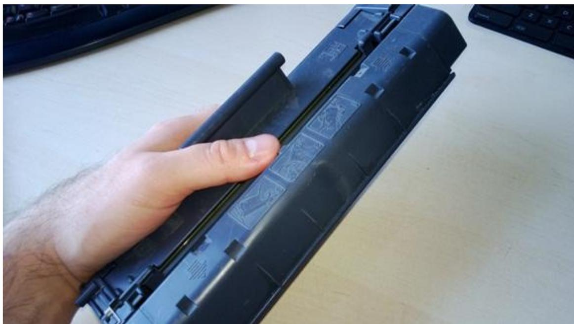
Most types of laser printer toner cartridges are full of a dry ink, fine enough to be electrostatically attracted to the paper during printing (the refined nature of the toner makes it potentially dangerous if inhaled).
