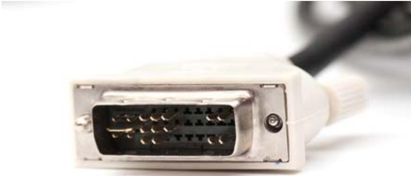
The DVI connection became the successor to VGA as technology moved away from analogue towards digital. Digital displays, like LCD, proved to be higher quality, which soon became the market standard for home pictures. DVI connectors come in 3 varieties.
