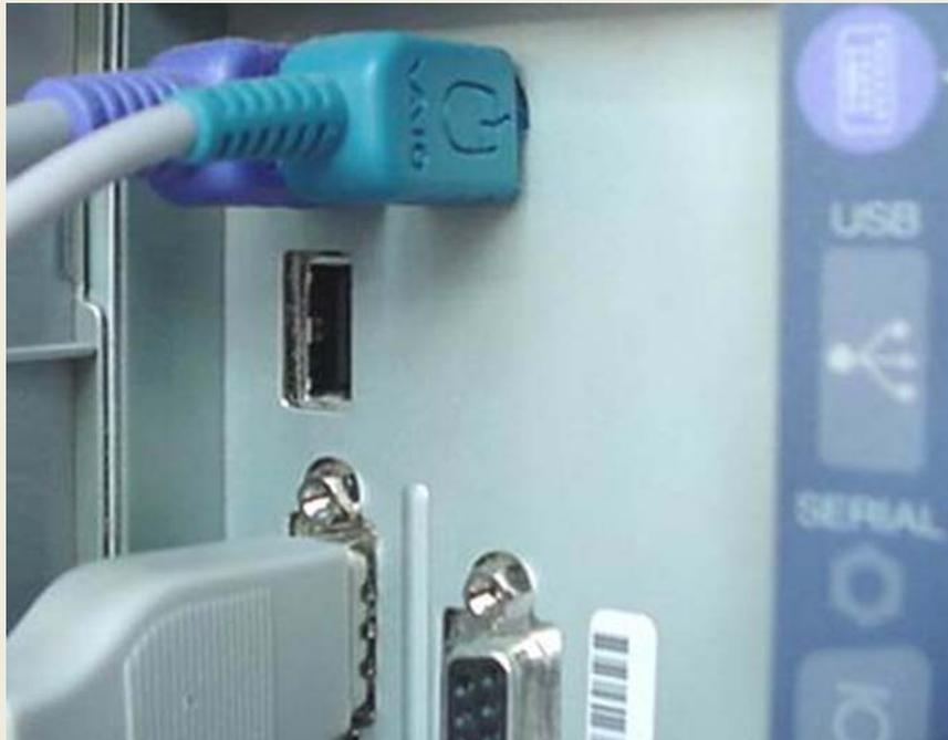
**The rectangular socket is a typical USB socket on the back of a PC**
