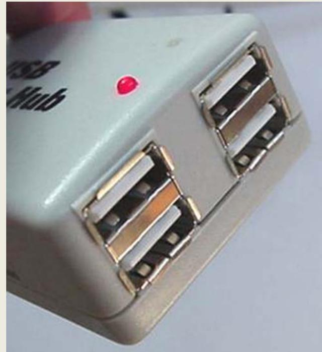
**A typical USB four-port hub accepts 4 "A" connections.**
