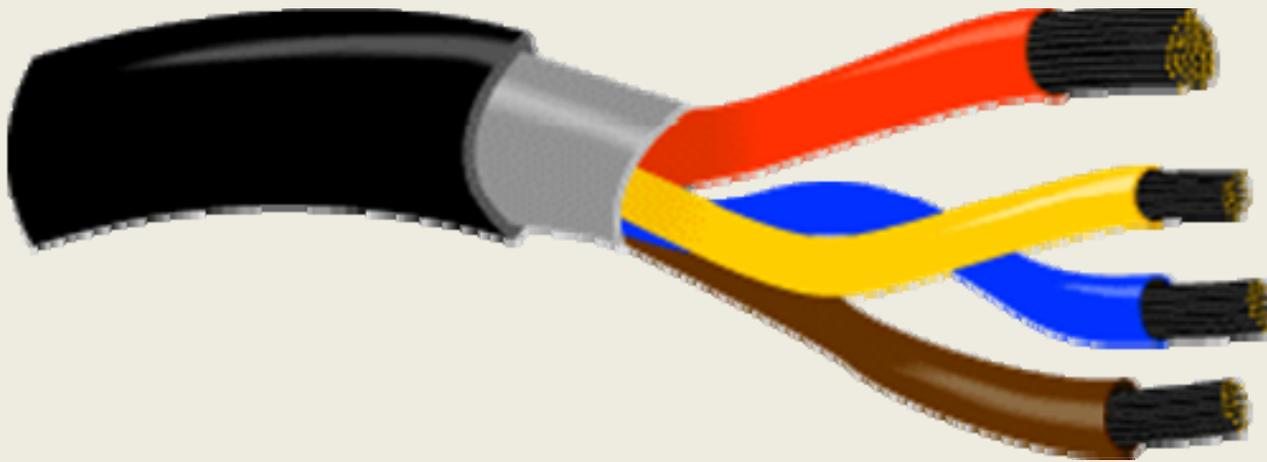
**Inside a USB cable: There are two wires for power – +5 volts (red) and ground (brown) – and a twisted pair (yellow and blue) of wires to carry the data. The cable is also shielded.**
